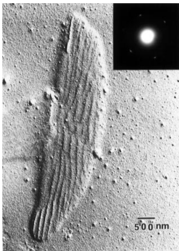
Figure 8. TEM observations of the TPP( n = 7 ) monodomain for the orthorhombic lateral packing grown on the amorphous carbon-coated surfaces. The ED pattern originates from the monodomain and is shown with the correct orientation.
